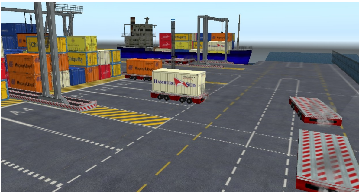
Illustration 2: ©Stessa IT Solutions, Container Terminal Simulation. You can see the Container Block Storage and the AGVs.
